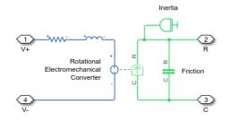
The following code implements the same model by means of a composite component, called DC Motor. The composite component uses the components from the Simscape Foundation library as building blocks, and connects them as shown in the preceding block diagram.
