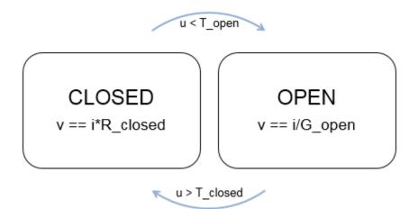
The following component implements the logic in the diagram by using a mode chart.
