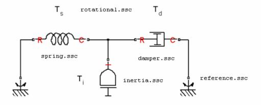
The domain is declared in a file named rotational.ssc (see "Declare a Mechanical Rotational Domain" on page 2-18). The following file, named spring.ssc, declares a component called spring. The component contains:
