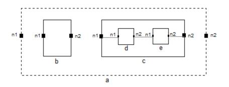
You are defining a composite component a, which consists of member components b and c. Component c is in turn a composite component containing members d and e. Each component has nodes n1 and n2.
